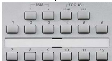
The control keys on the EKB200
